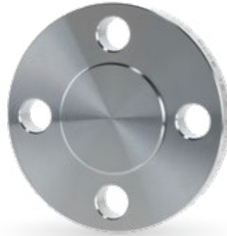
Blind - BL/RF Class 150 lbs, According to ASTM A182, ASME B 16.5
